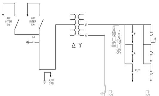
Figure 7. Unit Substation One-Line Diagram
