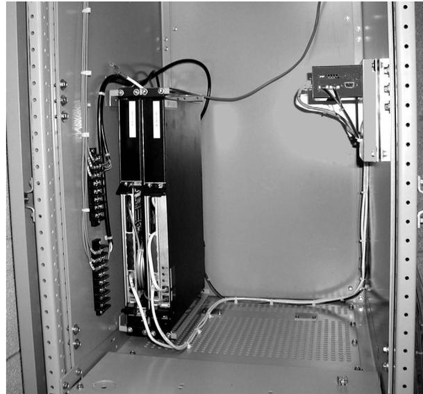
*Figure 4. Redundant Single-Processor Industrial Computers*
