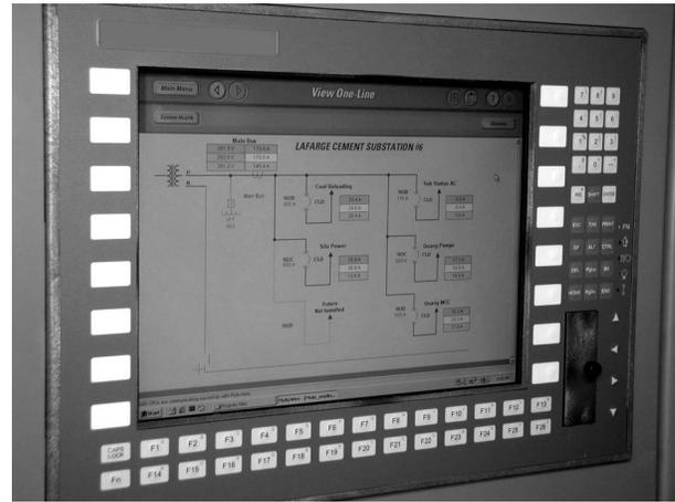
Figure 6. Human-Machine Interface (HMI) With Touch Screen
