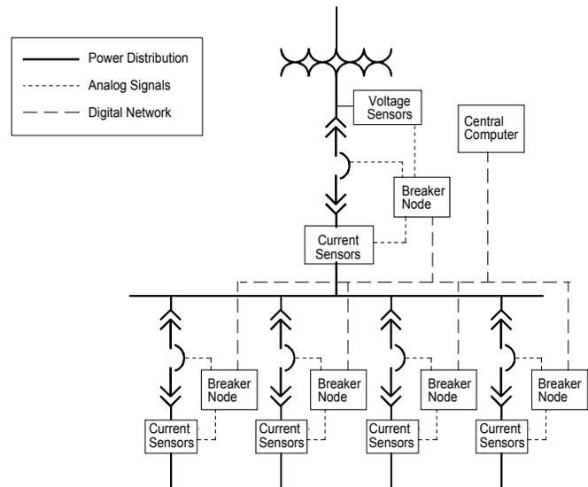
Fig. 1. Centralized architecture applied to a typical low-voltage switchgear lineup.
